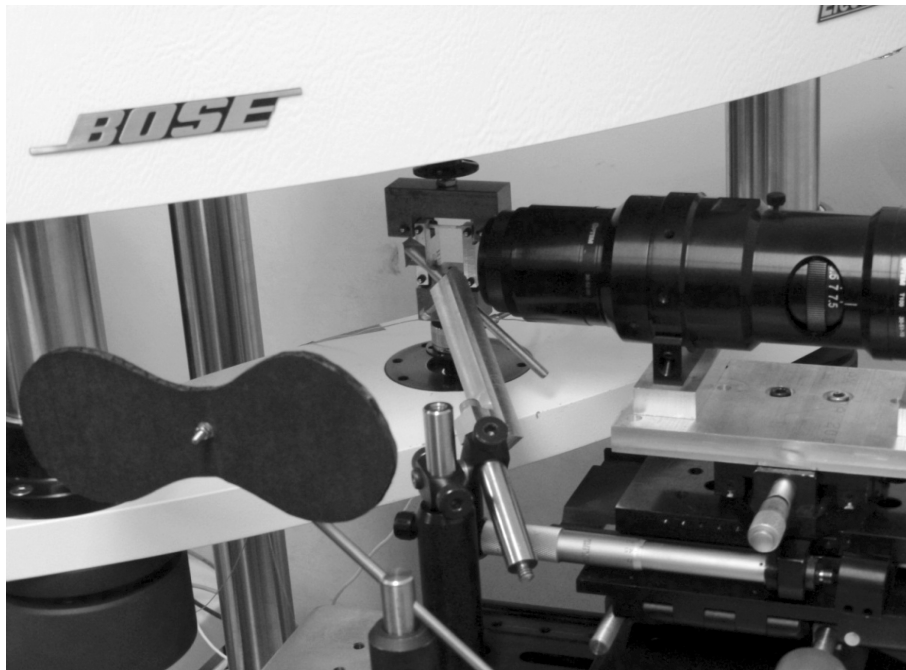
Figure 4: Sample and fixture installed in the Bose 3230 dynamic test machine.
